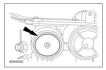
64. Using the special tools, install the retaining ring.
